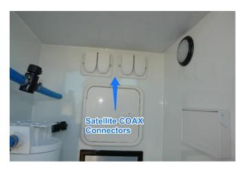
Of the two pairs of connectors, the right connector of each pair goes to the rooftop pre-wiring. The left goes to the living room or bedroom. If you have a rooftop installation, the rooftop connector must be jumpered to the living room or bedroom connector. The drawing below provides additional detail.
