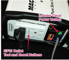
**NOTE:** After switching the battery cutoff switch ON, you must manually restart the inverter or the refrigerator will not receive any power from the batteries. If you are plugged into shore power while loading up for a trip, the refrigerator will run on 120V shore power. But if you forget to turn on the inverter, when you begin towing, the refrigerator will not receive power.
