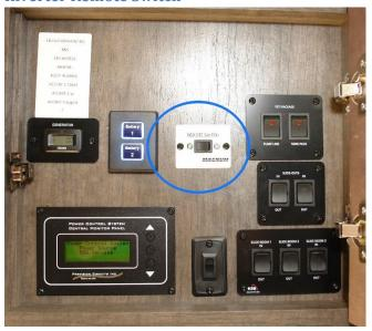
When towing, your batteries supply power to an inverter that converts 12V DC into 120V AC to power the Residential Refrigerator. Any time that 12V power is turned off, either by removing batteries for service or when in storage, or by turning the battery cutoff switch(es) or relays OFF, the inverter will turn off and stay off when power is reconnected. The remote switch may be used to turn the inverter ON, provided the battery cutoff switches or relays are ON.
