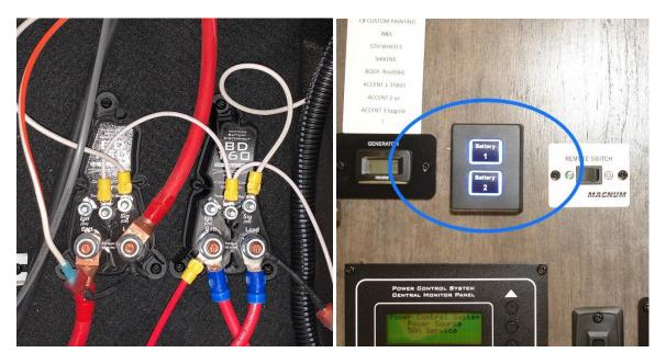
The control panel switches labeled Battery 1 and Battery 2 each control one of the relays in the front compartment. Contrary to the labels, each relay receives power from both batteries. So one of the
