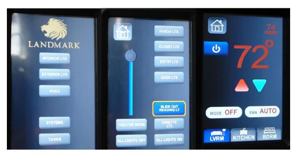
KIB Home Screen, Lighting Control Screen, and Thermostat with A/C and Heat Control
