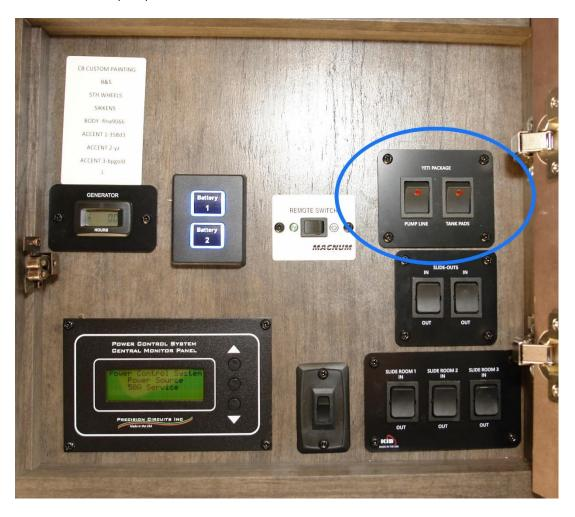
In sub-freezing weather, if the heat tape is not turned on before temperatures drop, you may have ice at the junction where the fresh tank drain hose is teed into the feed line. The water above the drain valve, and below the coroplast is first to freeze and ice can wick up into the tee fitting, blocking water flow.
