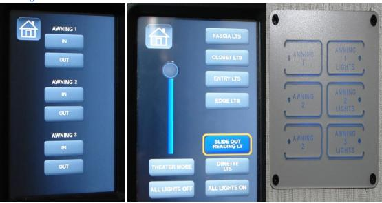
The Awning switch extends or retracts the awnings. Awnings may be controlled from either the KIB touchscreen, the phone app, or the local switches. The Awning Light switches turn on the LED strip mounted on the coach sidewall, along the awning.
