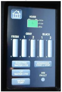
Use the KIB touchscreen or phone app to display the water level in each holding tank as well as the approximate voltage level of the 12V DC power system. Note that when plugged into shore power, the voltage reading reflects the higher of the battery level, output of the Power Converter, or the output from a connected tow vehicle. The Holding Tank Gauges give a very rough indication and can be affected by how level the coach sits, and other factors.
