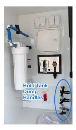
In floor plans with a 2<sup>nd</sup> bath, the pull handles may be arranged differently and the arrangement may vary by floor plan. Some handles may be located inside a separate compartment door near the UDC.
