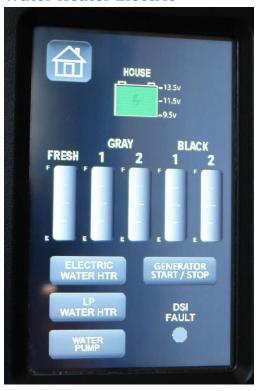
The dual-mode water heater can be operated in electric-only mode, LP mode, or both at the same time.
